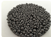
Fig. 3: A sample with steel hollow spheres of different diameters produced by Hollomet GmbH and bonded together using a resin adhesive.
