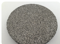
Fig. 2: A sample of sintered steel hollow spheres (globomet) produced by Hollomet GmbH.
